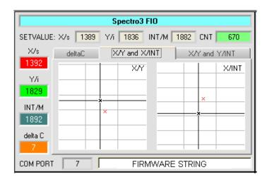
The X/Y and X/INT and the X/Y and Y/INT tabs provide a view of the current values of X, Y, and INT (or s, i, M) and of the SETVALUES of X, Y, and INT (or s, i, M) in two graphs.
